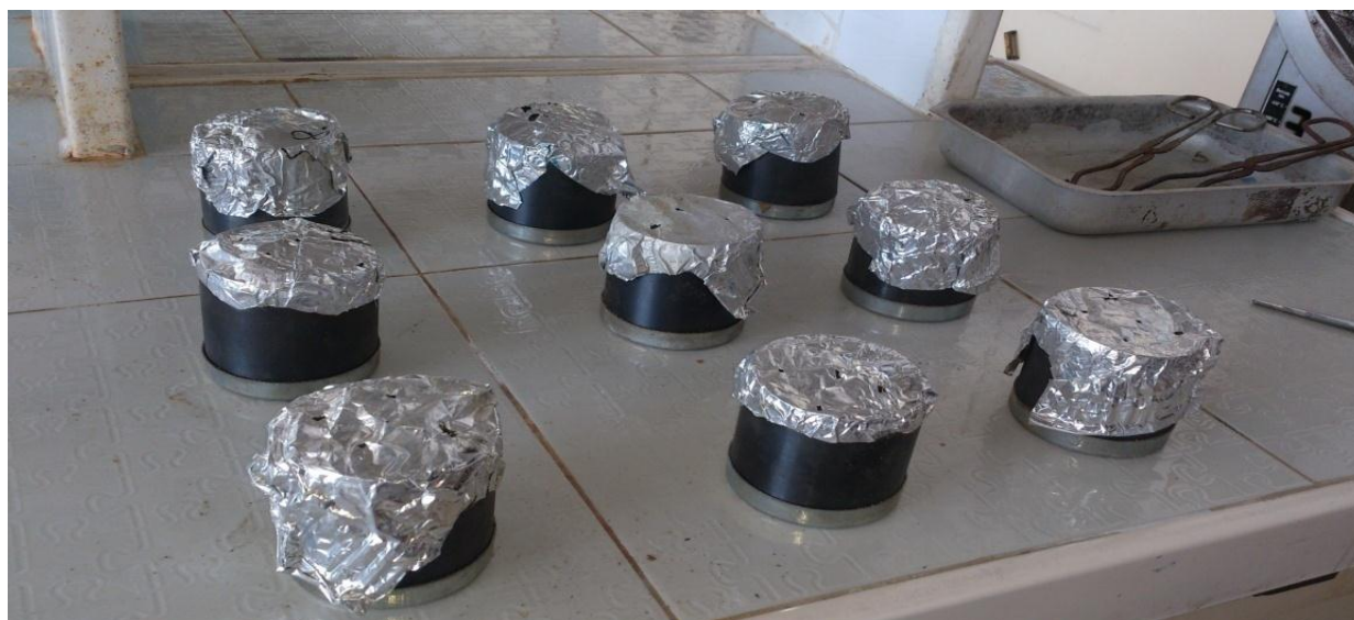
Picture 1: peanut pods samples in metal cylinders intended for carbonization.
